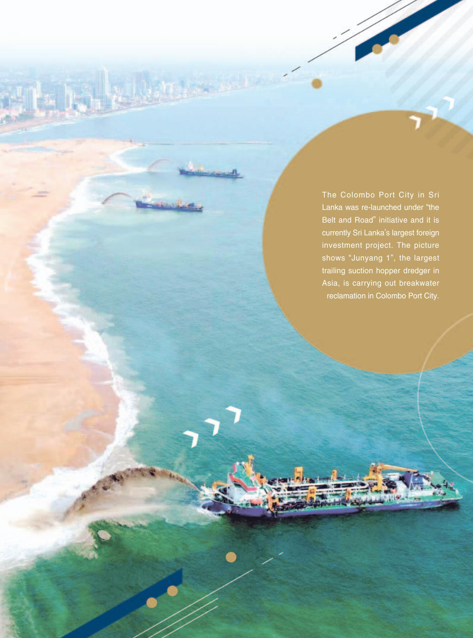
The Colombo Port City in Sri Lanka was re-launched under “the Belt and Road” initiative and it is currently Sri Lanka’s largest foreign investment project. The picture shows “Junyang 1”, the largest trailing suction hopper dredger in Asia, is carrying out breakwater reclamation in Colombo Port City.
